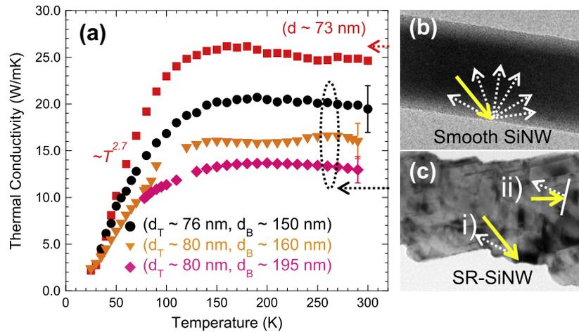
Fig. 7. Temperature-dependent thermal conductivity measurements of SR-SiNW. (a) Thermal conductivities as a function of temperature for smooth and SR-SiNWs. SEM images and schematic diagrams of phonon transport mechanisms in smooth (b) and SR-SiNWs (c).
