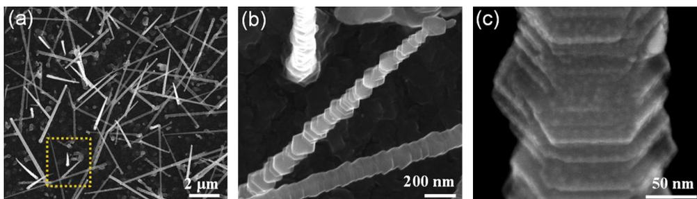
Fig. 3. SEM characterization. (a) SEM image of SiNWs grown on a 2 nm thick Au layer deposited on a Si(100) substrate using a hot-wall CVD system at 550 °C for 4 h. (b) Enlarged SEM image of squared region in (a). (c) HRSEM image of a SiNW showing the facets and Au NCs on the surface.
