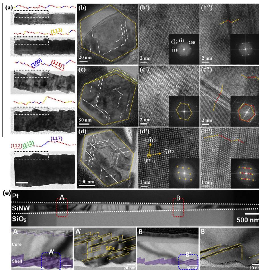
Fig. 5. Faceting and stacking faults analysis. (a) TEM images of SiNW facet orientations grown for 2, 3, 4, 6 and 9 h, respectively. (b–d) Quasi-6-fold cross-sectional TEM images of the SiNW grown for 3, 4 and 6 h, respectively. (b'–d', and b''–d'') HRTEM images of core and shell regions corresponded to (b–d). (e) Longitudinal TEM images of an individual SiNW grown for 4 h. (A–B') Enlarged images of squared regions.
