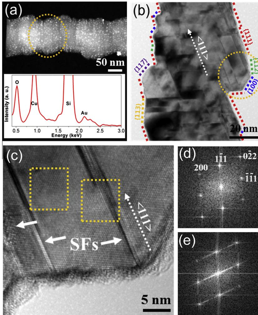
Fig. 4. TEM characterization. (a) STEM image and EDX spectrum of the bottom of a rough SiNW. (b) Bright-field TEM image of circled region in (a). (c) HRTEM image of squared region in (b). (d and e) Selected area electron diffraction patterns of squared region in (c).
