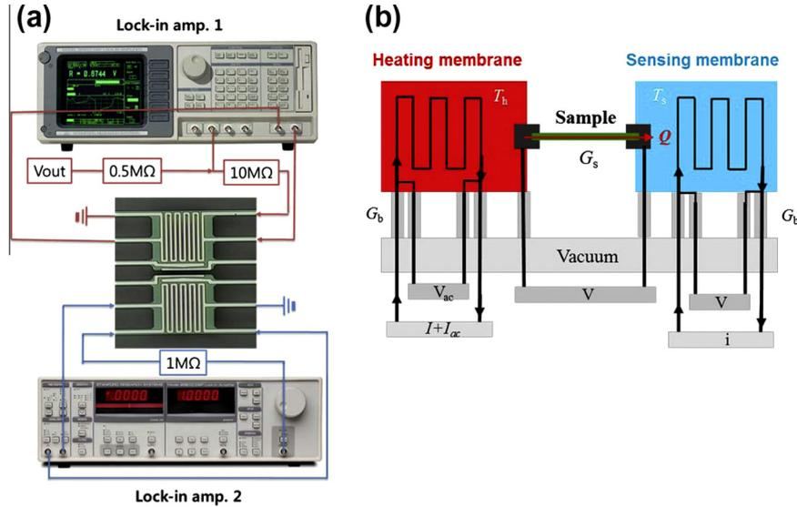
Fig. 2. Thermal conductivity measurement setup and thermal bridge method. (a) Schematic diagram of measurement setup for measuring the thermal conductance of the suspended SiNW using a microdevice chip. (b) Conventional thermal bridge method via a microdevice chip, which is composed of two suspended membranes. It indicates how to determine the thermal conductivity of SiNW suspended membranes.
